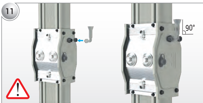
Open the plastic cover on the opposite side of the block joint to be cast, and install the CCR Block Joint Casting Level Control Plastic.
