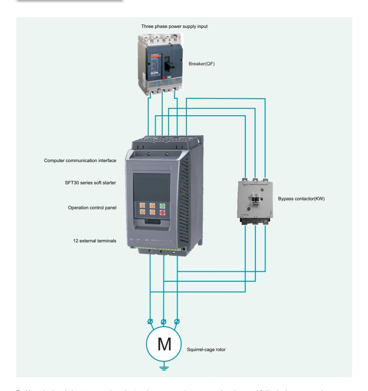
» Note: In the six input copper bar, the top three copper bar connect breaker, and followinghree copperbar connect bypass contactor.
