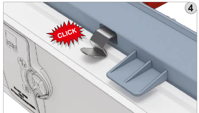
4 Be sure that the retaining springs are attached to the busbar
