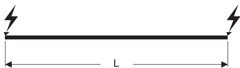
2 feeding points from the start points, L_t=L/4
